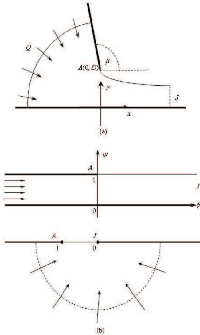
Figure 1: Sketch of the flow under a sluice gate (a) in physical  $z$ -plane, (b) in  $f$ -plane and artificial  $\zeta$ -plane.
