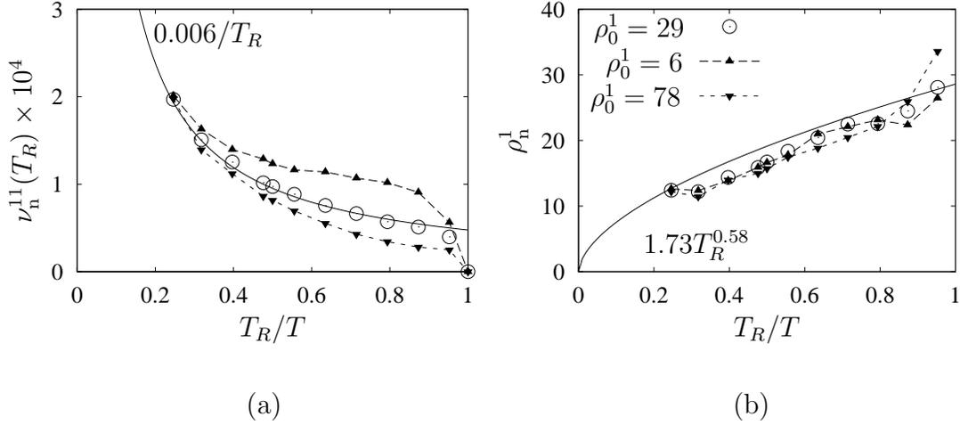
Figure 4: Using the T126 DNS data set, the sensitivity to  $\rho_0^1$  of the subgrid coefficients properties: (a)  $\nu_n^{11}(T_R)$ ; and (b)  $\rho_n^1$ , for various values of  $T_R$ . The legend in (b) also represents the data in (a).
