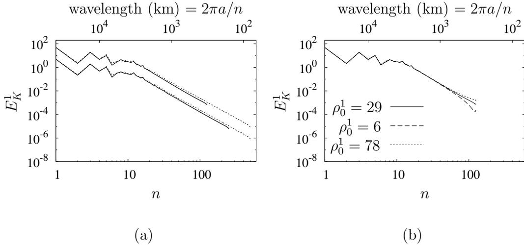
Figure 5: Comparison of the kinetic energy spectra on level 1 ( $E_K^1$ ) between: (a) the T504 DNS and the T126 DNS (top spectra), and with the T252 DNS (bottom spectra, shifted down one decade for clarity); and (b) the T126 DNS using three different power laws with  $\rho_0^j = 29, 6, \text{ and } 78$ .
