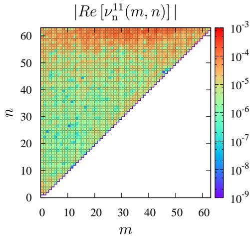
Figure 1: Net eddy viscosity subgrid coefficients  $|Re[\nu_n^{11}(m, n)]|$  required to truncate the T504 data set back to an LES data set with  $T_R = 63$ .
