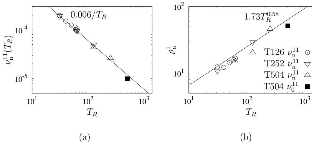
Figure 3: The scaling of the subgrid coefficients properties: (a)  $\nu_n^{11}(T_R)$ ; and (b)  $\rho_n^1$ , determined from three DNS data sets T504, T252 and T126 truncated back to various values of  $T_R$ . The legend in (b) also represents the data in (a).
